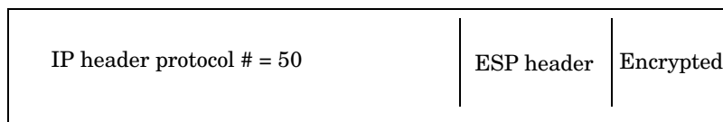
Figure 8-6 Packet with IPSec-Encrypted TCP Data
