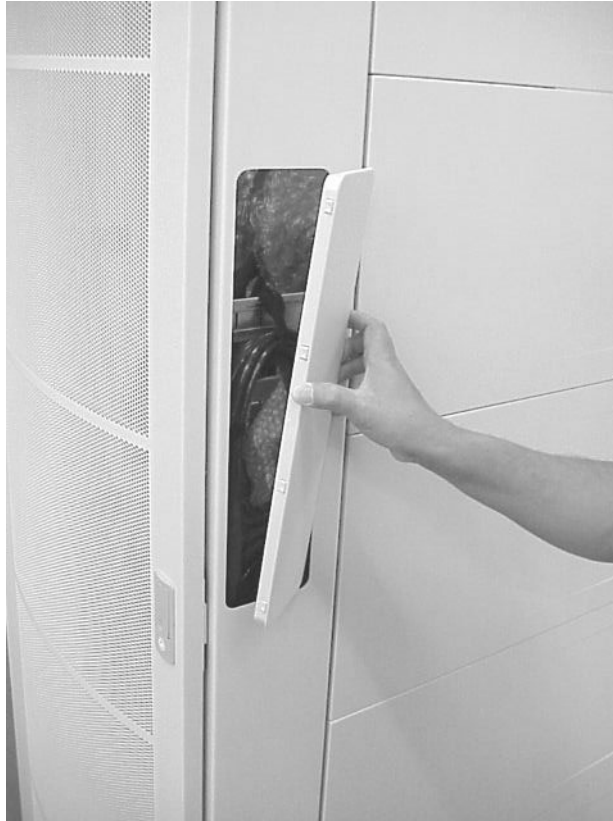
Figure 3-18 IOX Exit Cutout Blank Panel
