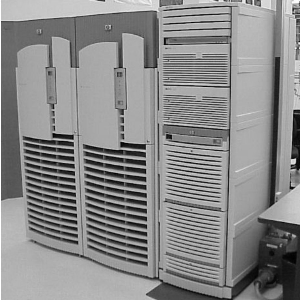
Figure 1-1 I/O Expansion Cabinet Shown With Superdome 64 Way
