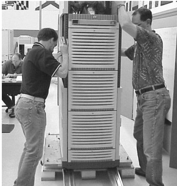
Figure 3-14 Rolling the IOX Down the Ramps
