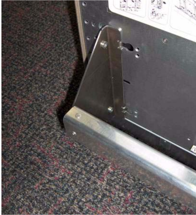
Figure 2-5 Inserting Rear Handle Tabs into Chassis
