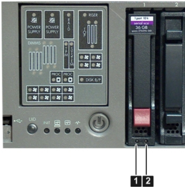
Figure 1-8 Hot-Pluggable SAS Drive LEDs
