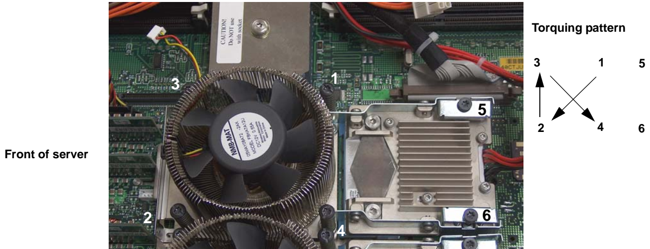
Figure 4-37 Secure the Captive Screws
