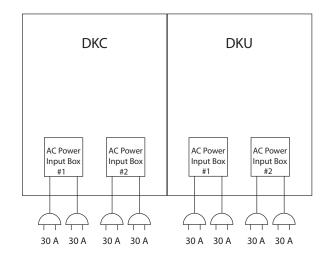
Be sure to install Russellstoll 3933 (alternate, 9C33U0) or 3753 (alternate, 39R33U0W) socket receptacles between the power distribution panel of the building and the attachment plugs for each unit.
