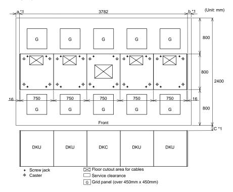
Clearance (a+b) depends on the floor load rating and clearance (c). The following table lists floor load ratings.
