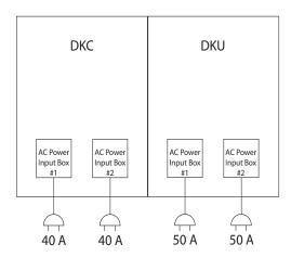
Be sure to install Russellstoll 9C53U2 or Russellstoll 9R53U2W socket receptacles between the power distribution panel of the building and the attachment plugs for the unit.
