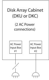
The Disk Array can tolerate the loss of connection to AC Box 1 or AC Box 2.
