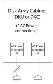
The Disk Array can tolerate the loss of connection to AC Box 1 or AC Box 2.
