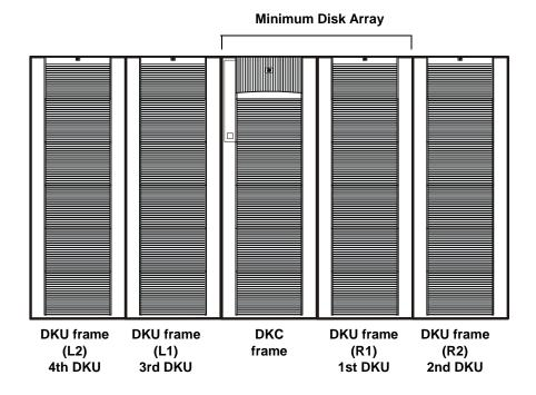
When both XP1024 and XP512 DKUs are used, the disk array can have one or two XP1024 DKUs (on one side of the DKC) and one to three XP512 DKUs (on the other side of the DKC) as shown in the figure below. XP1024 and XP512 DKUs cannot be mixed on the same side of the DKC.
