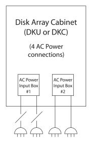
The Disk Array can tolerate the loss of connections to AC Box 1 or AC Box 2, but no other combinations are allowed.
