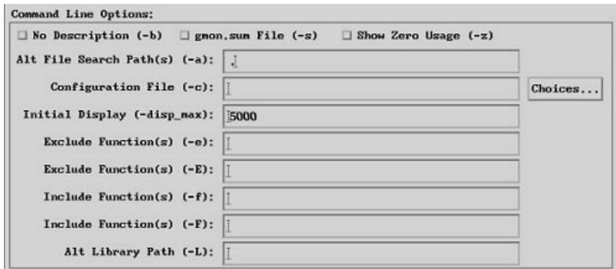
Figure 5. The Command Line Options area. The screen capture below is the Command Line Options box of the Load Files Dialog window. There are three check boxes side by side at the top: No description (-b), gmon.sum File (-s), and Show Zero Usage (-z). Below that, there are eight boxes corresponding to the eight Xprofiler GUI command-line flags, Alt File Search Paths (-a), Configuration File (-c), Initial Display (-disp_max), Exclude Functions (-e), Exclude Functions (-E), Include Functions (-f), Include Functions (-F), and Alt Library Path (-L), that are described in great detail below. There is a Choices button next to the Configuration File (-c) box.
