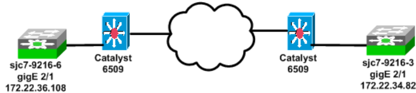
Figure 8-3 FCIP and IPsec Topology
