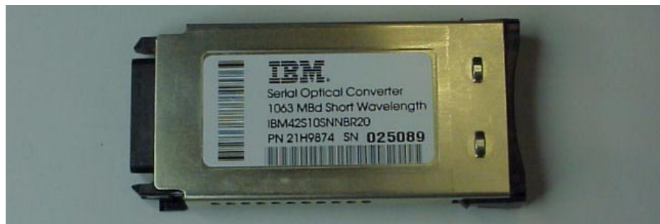
Figure 1-2 Short-Wavelength Laser (SWL) fiber-optic GBIC module
