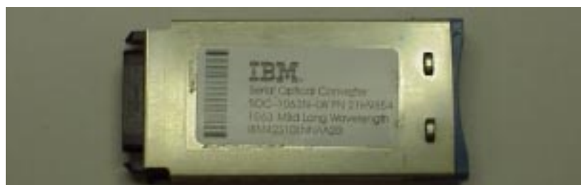
Figure 1-3 Long-Wavelength Laser (LWL) fiber-optic GBIC module
