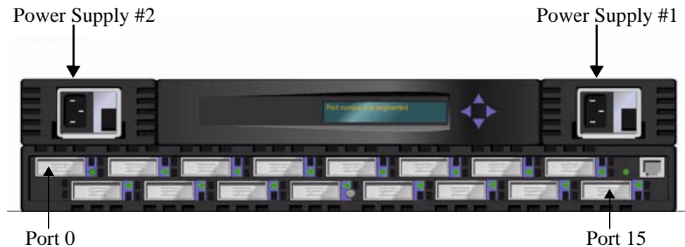
Figure 1-1 SilkWorm 2800 Front Panel
