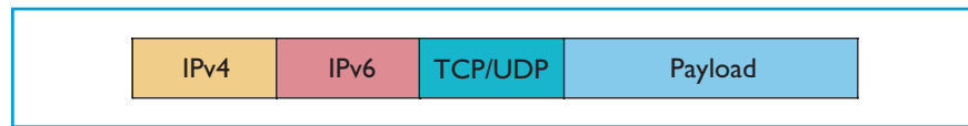
Figure 2. IPv6 in IPv4 tunnel. An IPv4 packet carries an IPv6 packet within its payload.
