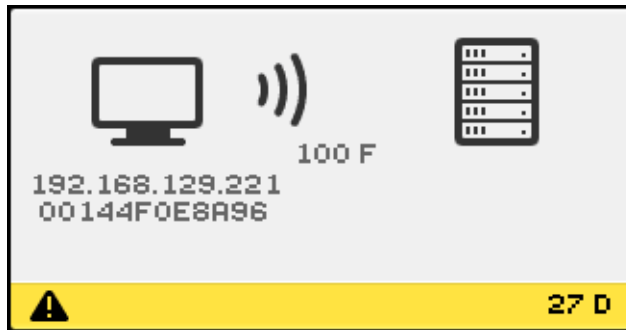
FIGURE B-12 DHCP Broadcast Failure
