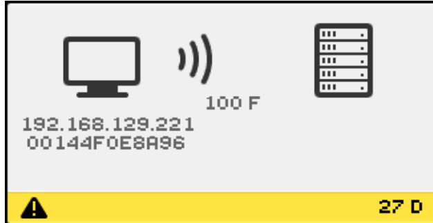
FIGURE B-12 DHCP Broadcast Failure
