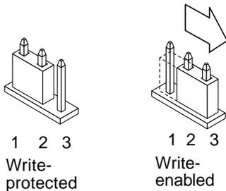
**FIGURE 1-12** Setting the Write-Protect/Enable Jumper to the Write-Enable Position
