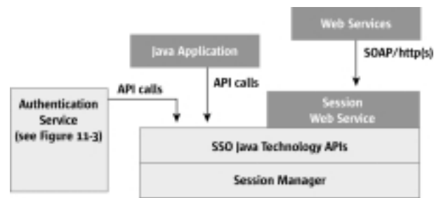
Figure 11-4: Web SSO Solution Architecture
