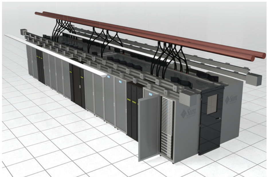
Figure 5. An architect's rendering of a pod that uses hot-aisle containment and APC InRow cooling systems on a slab or raised floor.
