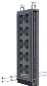
Figure 10. One cooling module accompanies each rack, with temperature-controlled fans modulating speed across five different zones.
